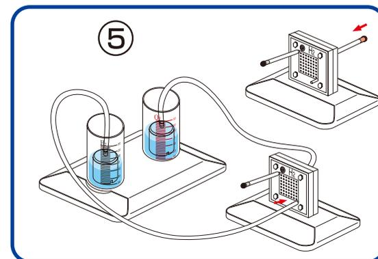
Procedure for repeated gas production: Reconnect the solar cell to the reversible fuel cell. Disconnect the small plugs from the tubes connected to the nozzles on the reversible fuel cell. This will allow water into the inner cylinders to replace the gasses and reset water levels to "0" line. Re-insert the plugs into the tubes and repeat electrolysis again.
