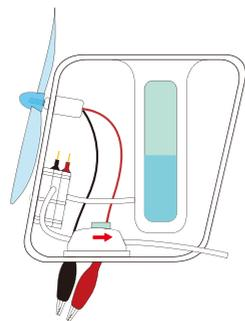
*Make sure the tubing connecting the tubing with purging valve is securely connected to the fuel cell and the switch on the purging valve is positioned at the right side close to the solution tank.*
