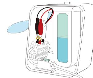
**If you have waited for 5-10 minutes with the clips disconnected from the fuel cell, the fan should start rotating by itself once connected. Make sure you repeat the waiting period of 5-10 minutes after each purging. Since the reaction is slow, the fan can run for up to several hours without purging (see Experiment 3).**
