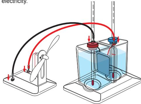
**Note:** At this moment, the temperature difference between the two sides should be more than 70°C. The temperature difference is proportional to the generated power. A 70°C difference of temperature is enough to power the fan for a long time. The power is generated due to Seebeck's effect which turns heat into electricity.
