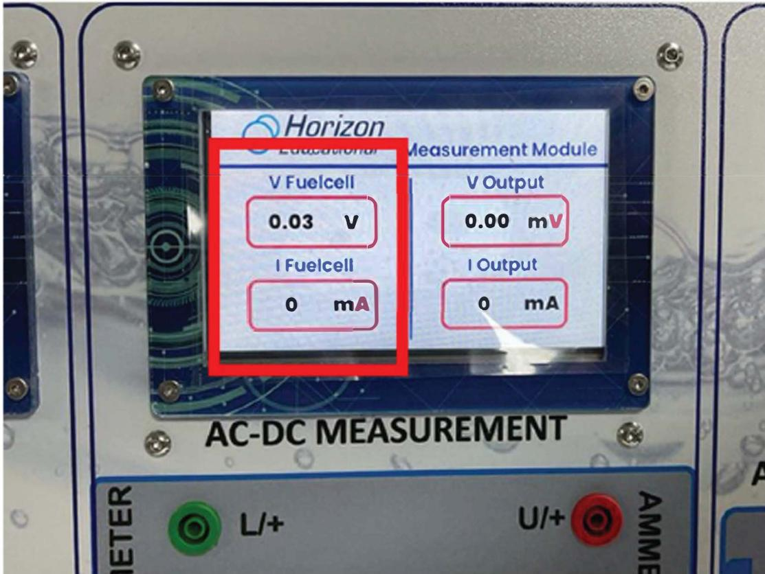
The output section measures the values of the binding posts on the DC measurement module.
